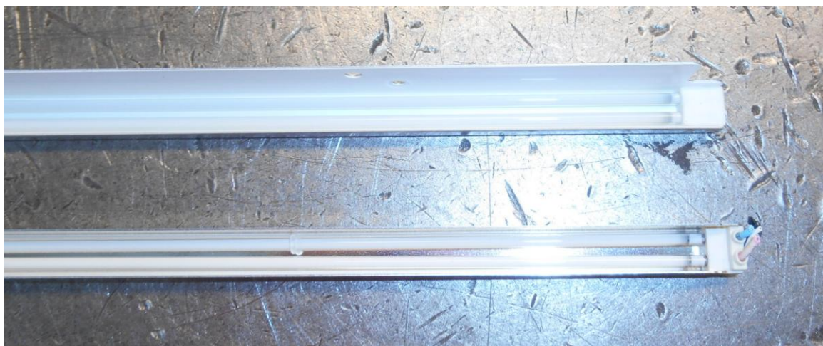
Picture 3.5.2.2: Backlight lamps including plastic/metal parts and covers:
