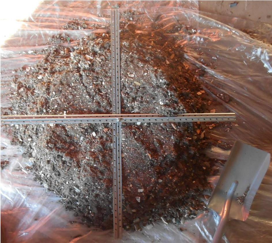
Portable sieve for sieving physically smallest non-metallic mechanical treatment fraction produced by the process in case of particles size over 5mm:
